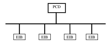
The EIB components are configured on the bus with the ETS tool. The corresponding PCD fonctions are programmed in Fupla using Fboxes of the EIB library.
