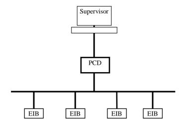
Using Receive Fboxes in the PCD, the actual state of sensor is always up to date in PCD variables. No pooling is necessary on the EIB Bus. The supervisor can read this values in PCD variables.
